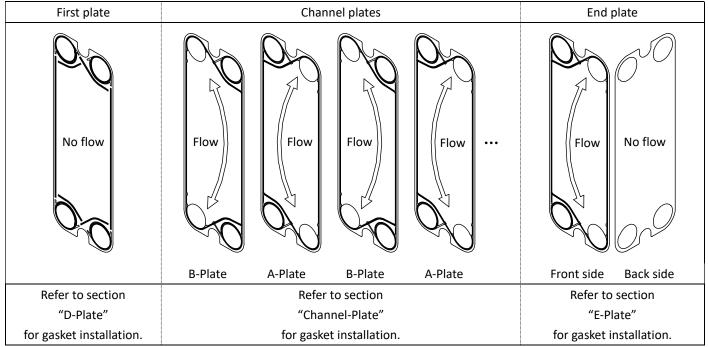
• Gasket has each type, style, size and setting position depend on PHE models.
