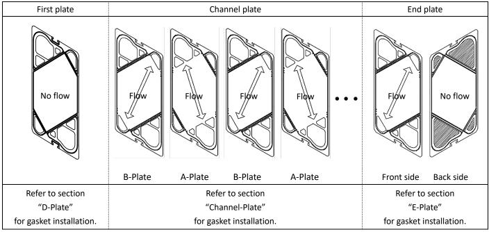
• Gasket has each type, style, size and setting position depend on PHE models.
