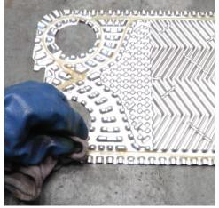
Photo 3. Removing work with a dust cloth
