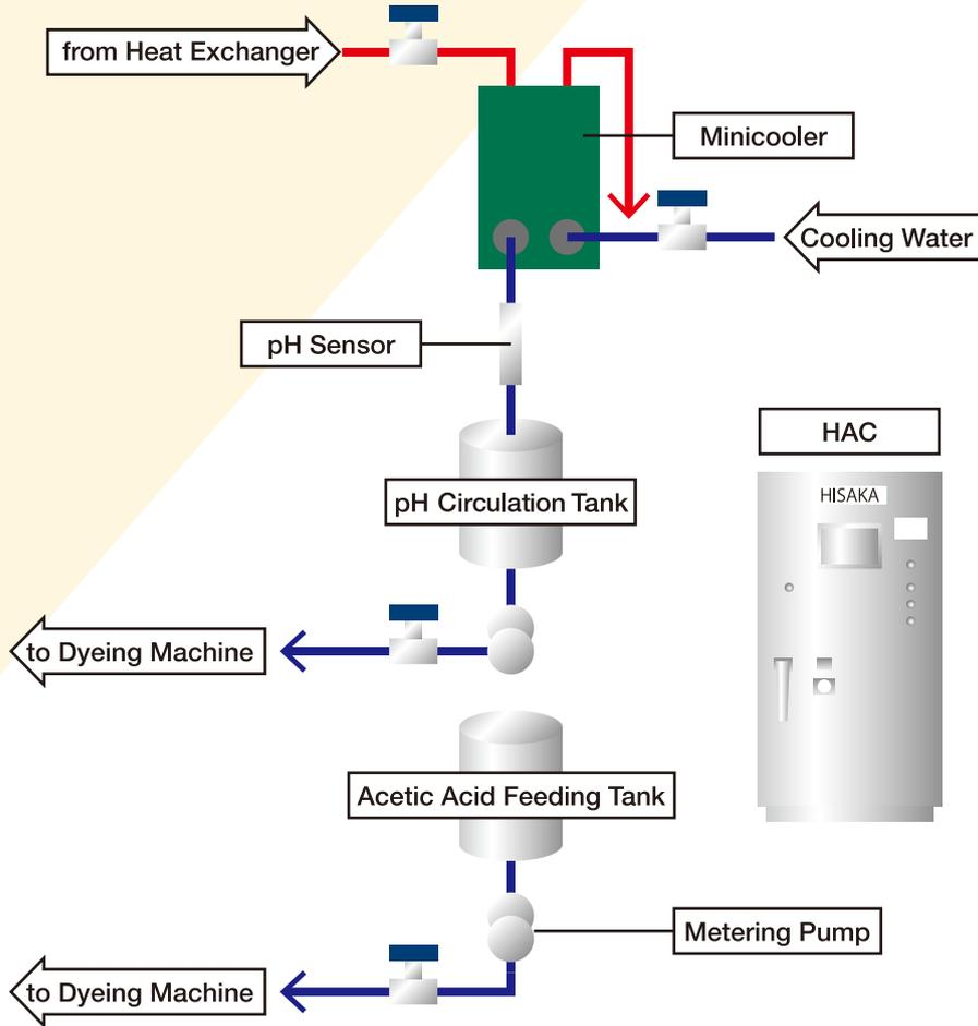
Control Device (HAC) controls pH value with continuously detecting the current pH value. The feeding volume and speed of Acetic Acid are controlled by Metering Pump.
