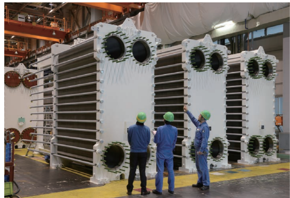
UX-160, one of the largest plate heat exchangers in the world
