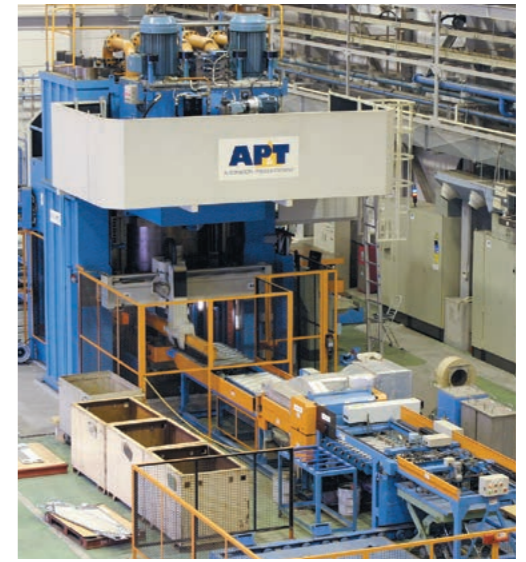
High-speed, automated 4,000 ton press
