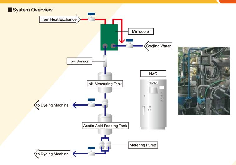
Control Device (HAC) controls pH value with continuously detecting the current pH value. The feeding volume and speed of Acetic Acid are controlled by Metering Pump.
