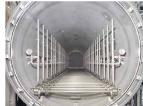
Inside the spray type sterilization tank
