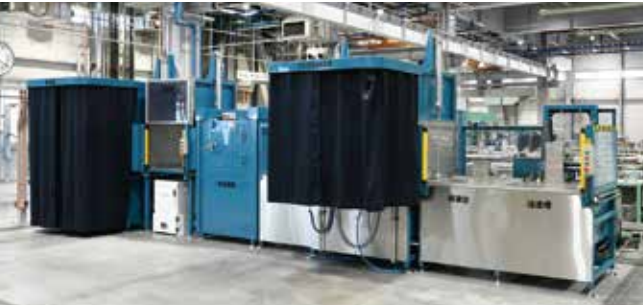
Valve Division Liquid penetrant testing equipment This system was introduced to improve the productivity of penetrant testing, which is a non-destructive inspection of high-pressure gas certified products and inspected products, and to improve the working environment.
