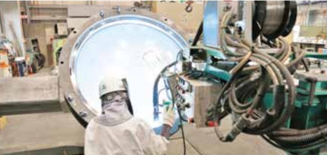
Process Engineering Division High precision automatic welding machine for stainless steel This high precision automatic welding machine plays an active role in making sterilization, disinfection and dyeing equipment. We were the first in Japan to develop and successfully apply this type of machine in the manufacturing of pressure vessels. It can also weld many high quality materials such as super stainless steel.
