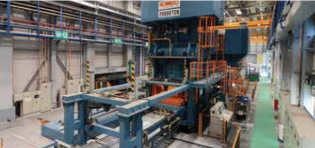
Heat Exchanger Division 20,000-ton automated press line This state-of-the-art totally automated, unmanned press line achieves productivity 1.5 times higher than previous lines. It can cope with plate sizes ranging widely from medium to large size.
