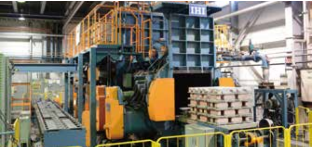
Heat Exchanger Division Continuous vacuum furnace This is one of the world's largest continuous vacuum furnaces, boasting a maximum processing load of 2,000 kg. It is used for brazing the brazed heat exchangers.
