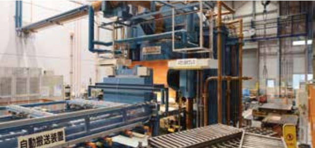
Heat Exchanger Division 40,000-ton automated press line This 40,000-ton automated press line - the largest class in the world - is composed of a forming press, crack detector and conveying devices. It produces various different types of large size titanium plates for use in LNG plants and similar.
