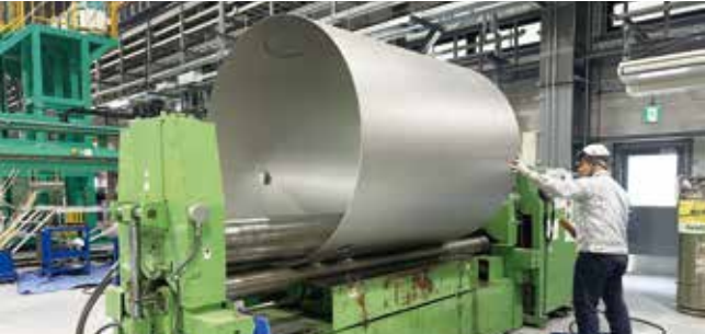
Process Engineering Division Bending rolls This equipment can accurately bend stainless steel plates of a wide variety of thicknesses. This bending technology, indispensable for fabricating sterilization, disinfection and dyeing equipment, supports our high quality products.
