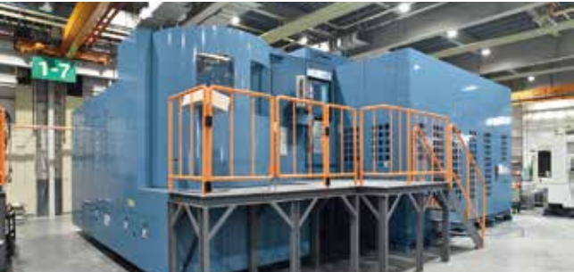
Valve Division 5-axis vertical type multi-functional machine This numerically-controlled multi-functional machine fabricates the main bodies of large size valves. It can machine multiple surfaces, eliminating useless work and enhancing dimension precision.
