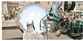
High precision automatic welding machine for stainless steel
