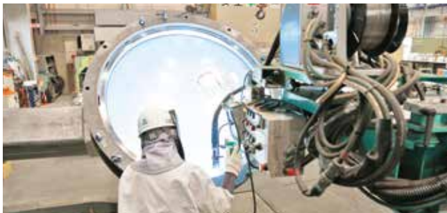
Process Engineering Division High precision automatic welding machine for stainless steel
