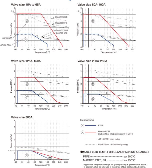
■Temperature and Pressure Rating for Low Temperature Ball Valve
