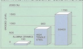
(TEST CONDITION:SPRAYING STEEL GRIT, SPRAYING 30DEGREE,PRESS 0.69MPa.TIME 60HOURS)
