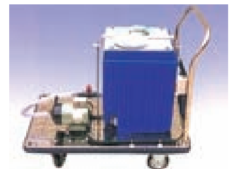
↑ Cleaning-in-place (CIP) Unit...A simple mobile CIP unit with caster wheels, and CIP cleaning for plate heat exchangers without disassembly.
