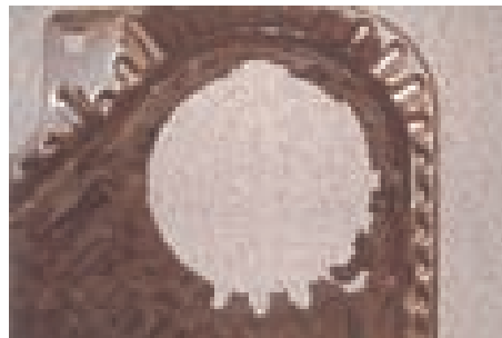
↑ Port hole of plating fluid side
