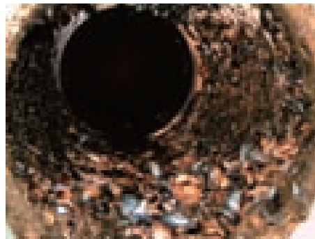
↑ Heat exchanger Seawater inlet port hole Wood chips, seaweeds and shellfish are blocking the flow channel, and causing poor flow in the unit.
